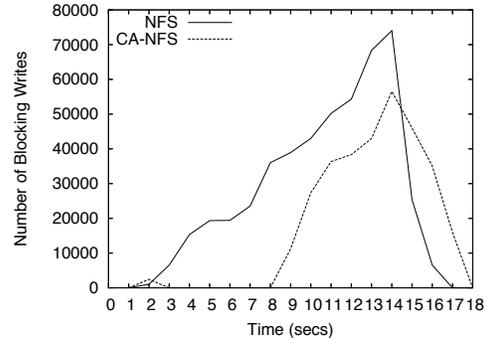
Figure 10: Number of asynchronous client writes blocked
