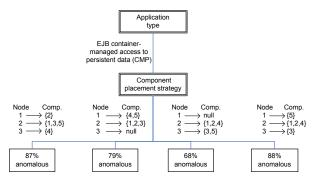
Figure 5: A three-level decision tree produced for debugging. Non-leaf nodes represent system configurations or workload conditions while leaf nodes represent decision points. The value inside each decision point indicates the likelihood of performance anomalies within that decision point's region. For brevity, we only show the decision points in the tree that are substantially anomalous.
