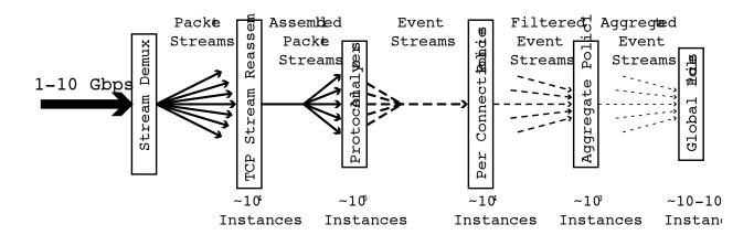
Figure 1: The spectrum of parallelism present in a high-level network security analysis pipeline.
