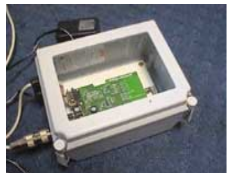
World Wireless Communications 900 SS 56kbps low cost radio, in field protection case.
