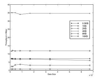
Figure 7. Client-Server Throughput for OmniORB on Linux
