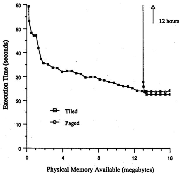
Figure 10: Performance of VM System on Filtering Task
