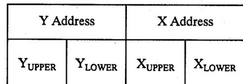
Figure 7: Anatomy of an Array Virtual Address
