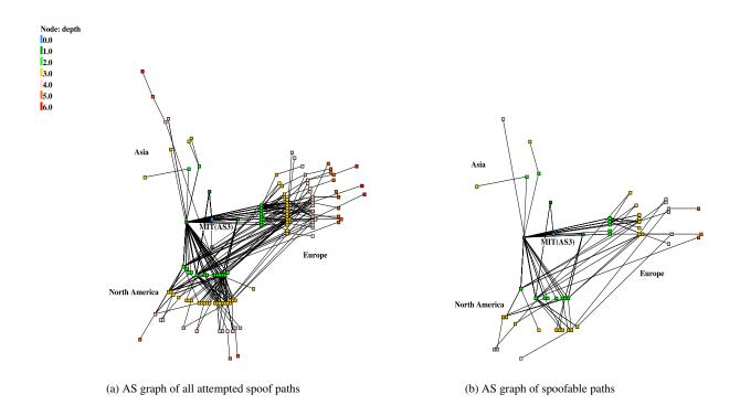
Figure 4: Visualizing geographic reach of spoofing. Each node represents an AS while edges show routing paths. The AS radius is determined by distance from our measurement host, degree by AS longitude. The graph of spoofable paths is a subset of all paths tested. Our server is in the center of the graph at depth zero.
