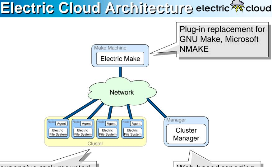
Inexpensive rack-mounted servers run pieces of build in parallel
