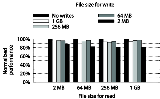
Figure 8: Zazen read performance under write workload. Writing data to the Zazen cache at a high rate (1 GB/s) does not affect the read performance in any significant way.
