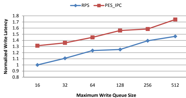
Figure 7: The write latency performance of RPS and PES_IPC while the maximum write queue size varies. Normalized to FIFO.
