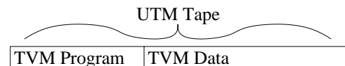
Figure 6: The tape of a Universal Turing Machine (UTM) stores the program and data of a hosted Turing Virtual Machine (TVM).
