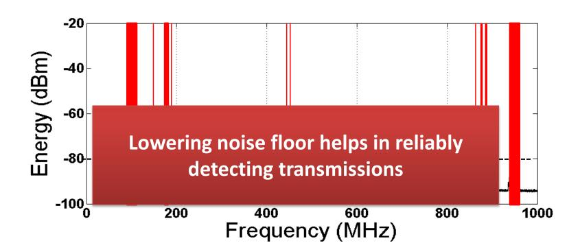
Noise floor determines the detection range of a spectrum analyzer
