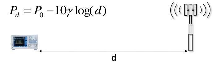
Lowering noise floor helps in detecting transmitters farther away
