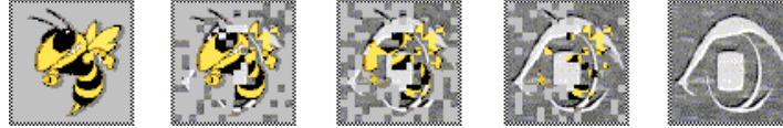
Figure 1: A time-lapse series of the fade widget for two images. Rather than perform compute-intensive calculations to achieve a fading effect, the original image is broken into pieces, and the pieces of the original are gradually replaced with pieces of the final.
