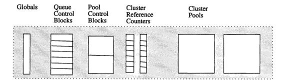
One side effect of multiple free pools is that the buffers need to be returned to the pools from which they were allocated in order to be coalesced into clusters. This is not difficult since each pool is composed of a
