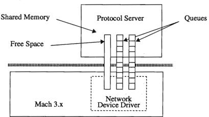
The design is derived from OSF/1 which, though a monolithic kernel, has a similar design. The network interrupt handlers communicate with the protocol threads by placing network buffers on appropriate protocol
