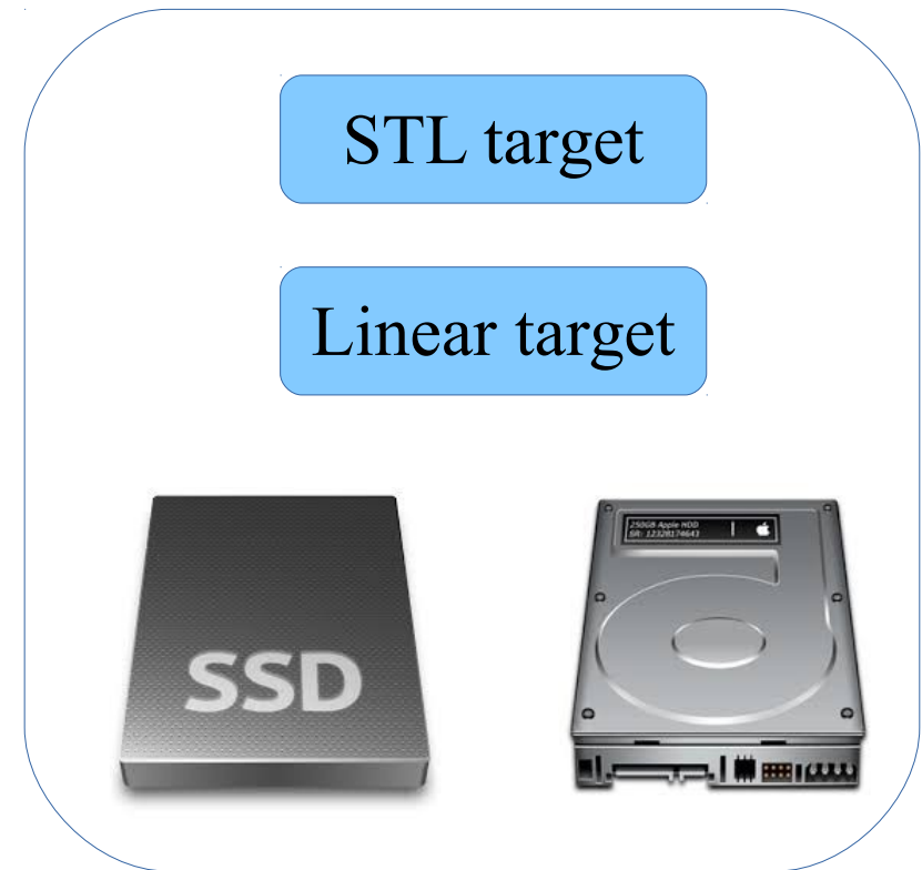
Drive-Managed SMR with persistent flash cache
