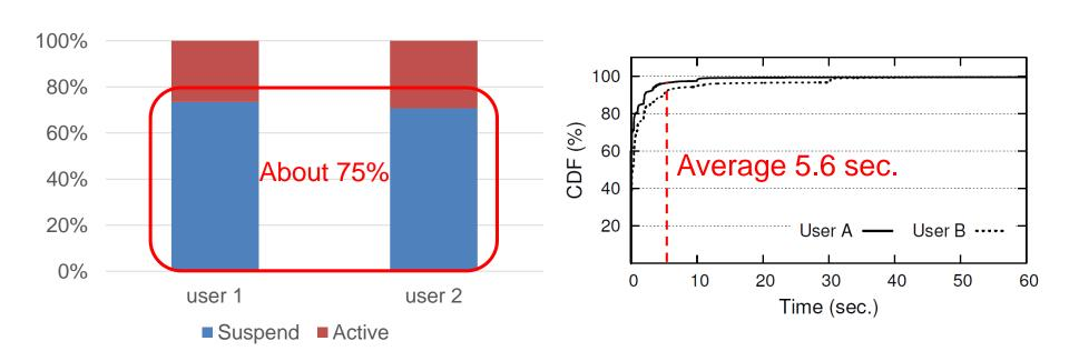
Device may be in suspend state when Background Segment Cleaning is activated.
