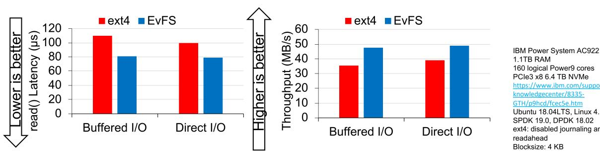
1.1TB RAM 160 logical Power9 cores PCIe3 x8 6.4 TB NVMe https://www.ibm.com/support/ knowledgecenter/8335-GTH/p9hcd/fcec5e.htm Ubuntu 18.04LTS, Linux 4.17 SPDK 19.0, DPDK 18.02 ext4: disabled journaling and readahead Blocksize: 4 KB
