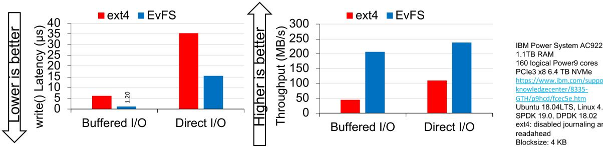
1.1TB RAM 160 logical Power9 cores PCIe3 x8 6.4 TB NVMe https://www.ibm.com/support/ knowledgecenter/8335-GTH/p9hcd/fcec5e.htm Ubuntu 18.04LTS, Linux 4.17 SPDK 19.0, DPDK 18.02 ext4: disabled journaling and readahead Blocksize: 4 KB
