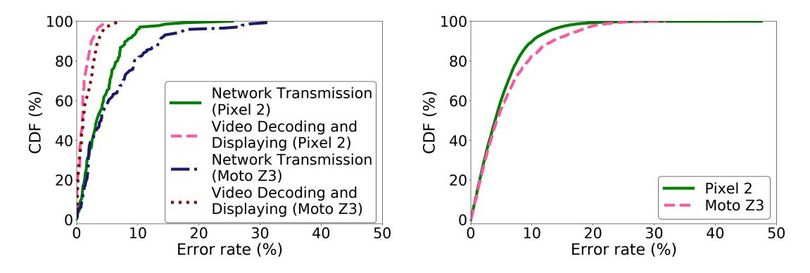
Function-wise power predictor achieves low mean per-interval energy prediction error of 4.87% (Pixel 2) and 5.86% (Moto Z3).
