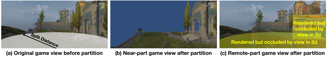
Figure 5: Three different game views in distance-based game partitioning. GPU usage overhead mainly comes from the occluded objects that are rendered in the remote game view (c) while not displayed in the original game view (a).
