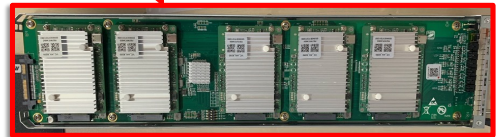
A Internal PCB board with 5 SoCs
