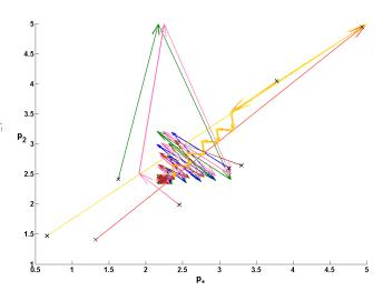
Figure 6: Trajectories of the best-response iterated play from different initial supplier prices (indicated with a cross symbol) for the example out-tree network with  $a_1 = 0.002$  and  $a_2 = 0.004$ . All the trajectories exhibit limit-cycle oscillations.
