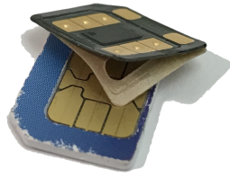
Figure 1: An overlay SIM (top) and a regular SIM (bottom). The top part of the overlay SIM can be peeled off and stuck on top of a regular SIM
