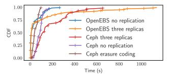
Figure 7: CDF of snapshot creation times for different storage provider configurations.
