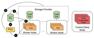
Figure 1: Basic topology of a Kubernetes cluster, with a single control plane node, multiple worker nodes, and a storage provider which aggregates local storage attached to each worker node. Also shows the operations and resources involved in providing a Pod with storage.
