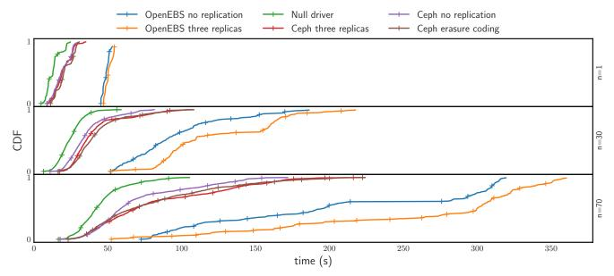
Figure 4: CDFs of time required to create and attach volumes for different storage provider configurations. n is the number of simultaneous volume creations. For all storage configurations, increasing the number of simultaneous volume operations increased the average time to create and attach an individual volume.
