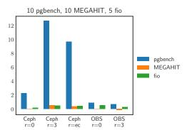
Figure 8: Change in performance compared to baseline, for three different ratios of I/O workload on five different storage configurations.
