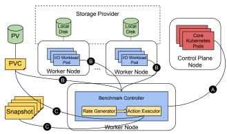
Figure 2: CNSBench overview with its components in blue
