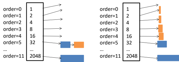
Figure 9: Allocation procedure of buddy system for 2 free pages.
