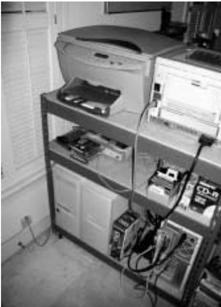
Figure 1: eden's core systems "neatly" arranged on over-the-counter shelving. Left to right: 300MHz Celeron rgb.adsl.duke.edu/adam (the gateway, note DSL plug on the wall), 466MHz Celeron abel, and dual 466MHz Celeron lucifer. The switches and so forth are on the middle shelf, printers on the top.
