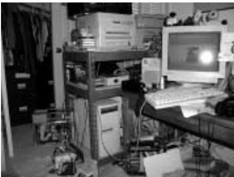
Figure 2: The front-end arrangement of eden. The monitor is connected to lucifer (left bottom), a dual 466MHz Celeron. Note KV switch
