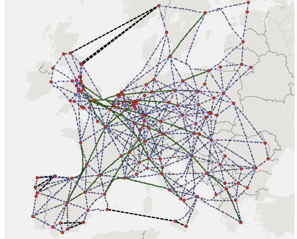
Fig. 13: A 100 Gbps 1.04\times stretch cISP across Europe. This network uses several fiber connections (dashed, black lines).
