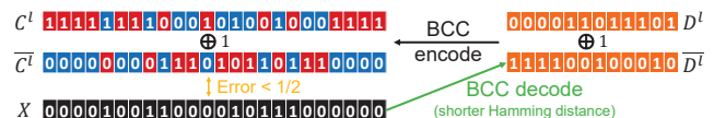
Figure 22: An example of the BCC decoding with complementary codewords at 1/2 coding rate.
