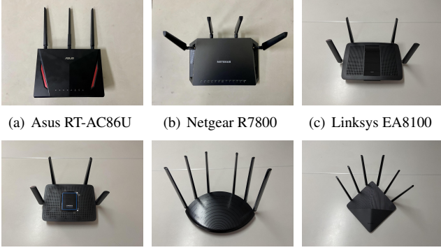
(a) Asus RT-AC86U (b) Netgear R7800 (c) Linksys EA8100 (d) Linksys MR9000X (e) TP-LINK WDR7660 (f) TP-LINK WDR7661 Figure 10: All tested routers support MU-MIMO technology.
