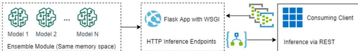
Figure 1: FlexServe architecture consists of an ensemble module which loads N models into a shared memory space. Inference output of each model is combined in a single response and returned to the requesting client as a JSON response object. The Flask application invokes the fmodels module, which encompasses the ensemble of models, and exposes RESTful endpoints through the Web Service Gateway Interface. Variable batch sizes provide for maximum efficiency and flexibility as clients are not restricted to a fixed batch size of samples to send to the inference service. Additional efficiency is achieved through the use of the shared memory, better utilizing available GPUs and requiring only one data transformation for all models in the ensemble.
