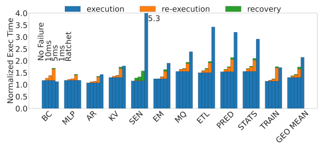
Figure 8: Latency overhead with power failure on MSP430
