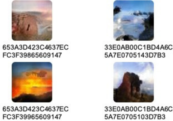
Figure 1: Sample key hashes, shown in hex format broken across two lines, that differ in a single bit (top and bottom) and their corresponding CEAL generated images. Unlike the textual keys, the images are easy to distinguish by humans.
