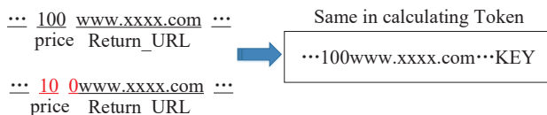
Figure 5: An example of the string shift in the order packet.
