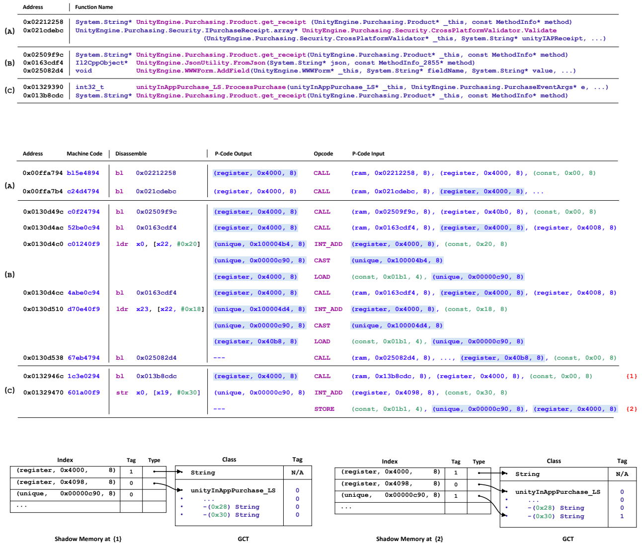
Figure 5: The Excerpt of the Disassembled Code, the Corresponding P-Code, and the State of Our Shadow Memory.
