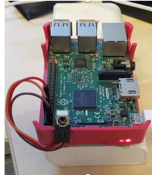
(a) IR Sniffer on Raspberry-Pi 3
