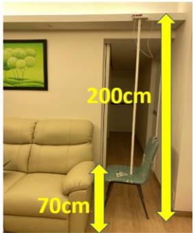
(b) Setup of IR sniffer
