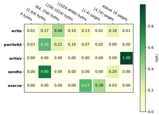
Figure 8: Heatmap showing the total amount of user data fetched by fetch-heavy syscalls.
