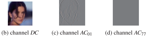
Figure 3: After block discrete cosine transform (BDCT), different visual information in the image is arranged in a zigzag pattern from low to high frequency. (b) (c) (d) represent the visual information in frequency channel DC , AC_{01} and AC_{77} .
