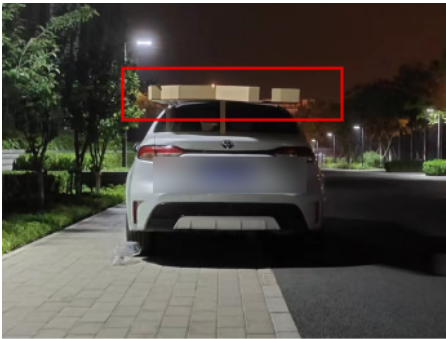
Figure 15: The adversarial ornament is placed on the roof of the target vehicle.
