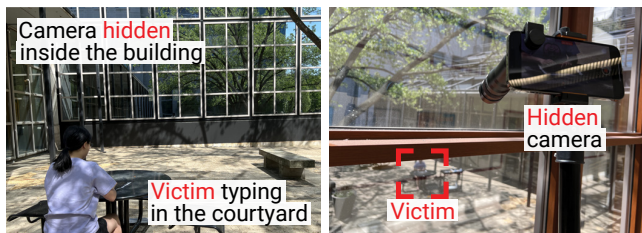
Figure 6: The experimental setup of our long-range, through-glass attack. The attacker videotapes the victim’s hands, by placing a smartphone camera with a budget telephoto lens inside a nearby building’s 2nd floor, behind the glass.
