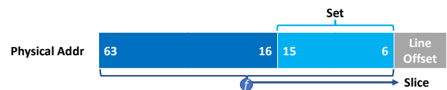
Figure 20: LLC slice and set function of i7-7700. The slice function ( f ) is a hash of certain bits from bits 6 to 63 while the set number is the linear bits 6 to 15.
