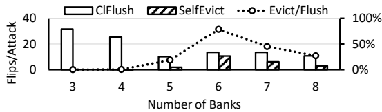
Figure 19: Rate of Flips compared between using cfluses (white) and Sledgehammer (striped). The number of flips Sledgehammer generates compared to cfluses (Evict/Flush) is shown in dotted lines.
