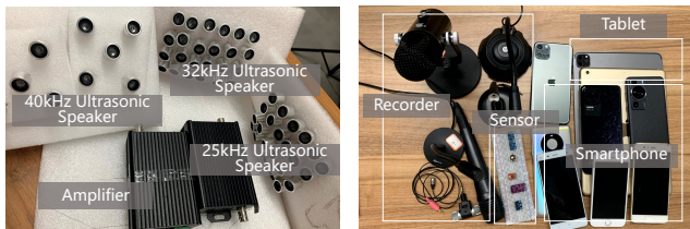
(a) The setup of ultrasound attack. (b) Victim devices. Figure 3: The experimental setup of ultrasound attacks is used and the targeted devices including smartphones, tablets, recording microphones, and sensors are tested in this paper.
