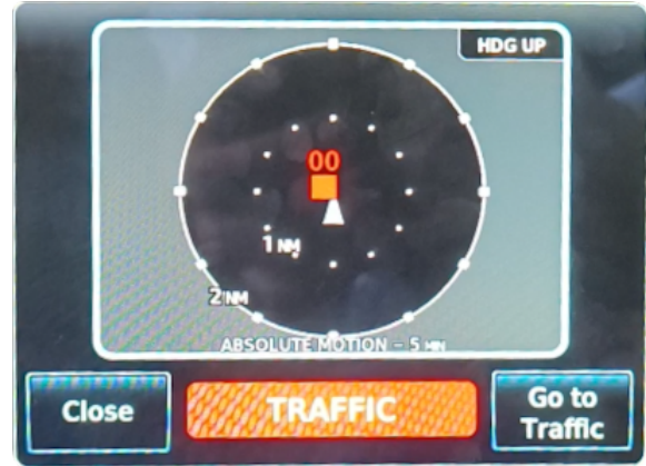
Figure 5: Avionics displaying a Resolution Advisory.
