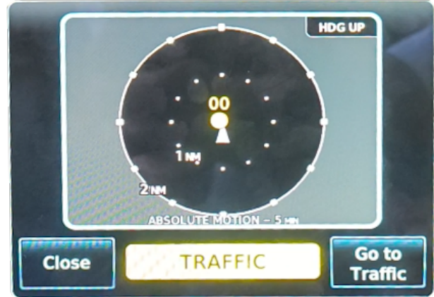
Figure 3: Avionics displaying a Traffic Advisory.
