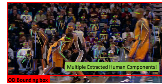
Figure 14: A common false positive case in sports tracking, where a crowd of people not in camera focus will be extracted as one bounding box by OD but have multiple components extracted. These cases are uncommon in the safety-critical domains of autonomous driving and surveillance due to the use of focus-free cameras.
