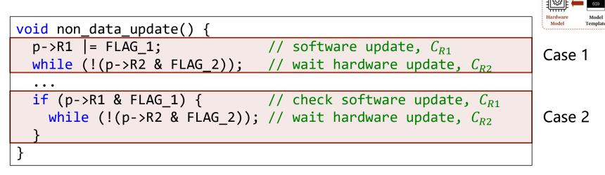
Software Belief: The value of register  $R_2$  must satisfy constraint  $C_{R_2}$  after the value of register  $R_1$  is updated in a way that constraint  $C_{R_1}$  is satisfied Hardware Behavior: Hardware updates  $R_2$  such that  $C_{R_2}$  is satisfied when  $R_1$  is updated in a way that constraint  $C_{R_1}$  is satisfied
