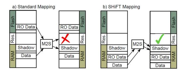
ASAN Mem-to-Shadow (M2S) : (Addr>>3) + Offset Incompatible with MCU (Muench et al. 2018)
