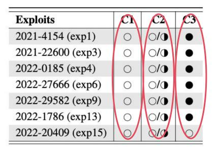
Hardenings in C1 are widely bypassed In C2, KFENCE can isolate only 0.005% -0.35% target objects; Securely storing random seed is challenging in structure layout randomization
