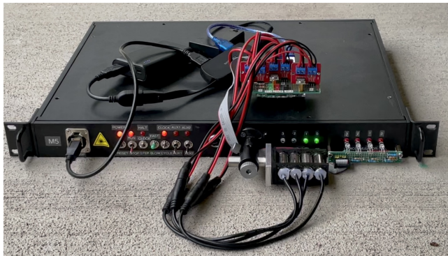
Figure 16: The M5 computer. Four lasers controlled by an Arduino with MOSFET laser drivers, are mounted aimed at the bus LEDs. The four LEDs on the right are the accumulator (A) register and the LEDs and switches on the left are used to interact with the computer.
